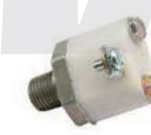
KRB279416 Low Pressure Indicator 1/4" P.T. Normally Open at 0 PSI Closes at 60 PSI
