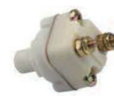
KRB228600 Stop Light Switch 1/4" P.T. Normally Open at 0 PSI Closes at 5 PSI
