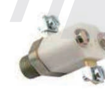
KRB228750 LP-3 Low Pressure Indicator 1/4" P.T. Normally Open at 0 PSI Closes at 66 PSI
