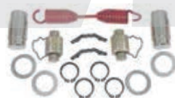
KRB-K1816 Universal Kit for Rockwell 16-1/2, Brake Standard. Includes: 2 roller, 2 roller retainer, 1 shoe return spring, 2 return spring pin, 4 anchor pin lock ring, 2 anchor pin, 4 anchor pin washer
