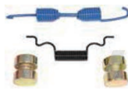
KRB-K5139 Universal kit for Eaton 15" x 4" EB & ES Front Brake Includes: 2 rollers, 1 shoe retainer spring, 1 return spring
