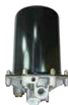
KRB65225D Air Dryer AD-9 12 Volts W/O Bracket Control Port 1/4" P.T. Supply Port 1/2" P.T. Delivery Port 1/2" P.T.
