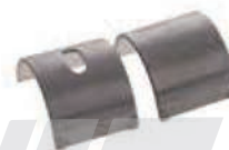
KRB107651 Connecting - Rod Bearing For TF550-STD
